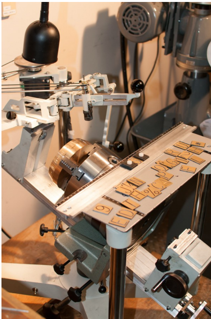
Engraving text around the circumference of the marker
