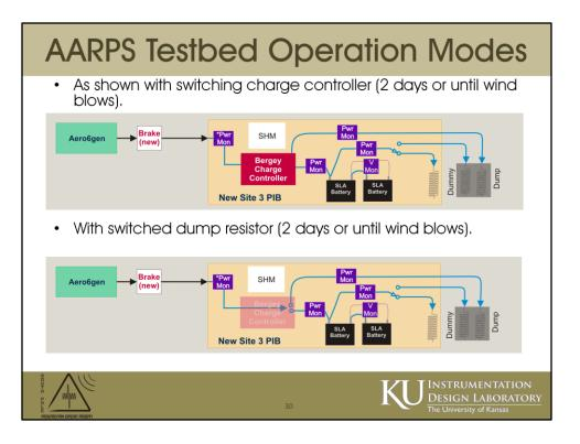
Connect the Aero6gen cable into the brake box and mount the dummy/dump resistor panel. (Were we using the one from WT2 for that?)
