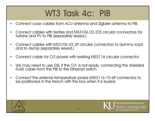
Ferrites: There are 2 sizes. Snap on one of each at each end of a run. Wrap with driller's tape (I hope there is some!) so they don't fall off.
