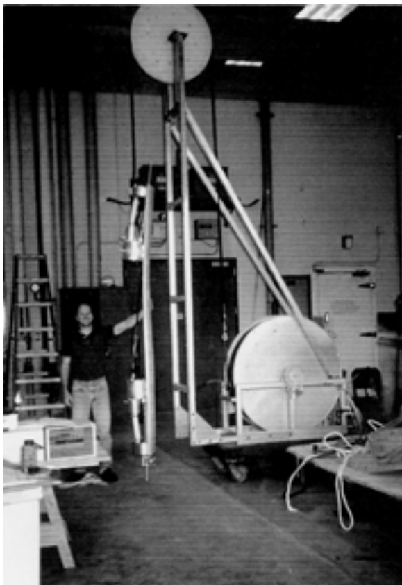
Figure 8. 2.5-m operational collector suspended from the cable on a winch.
