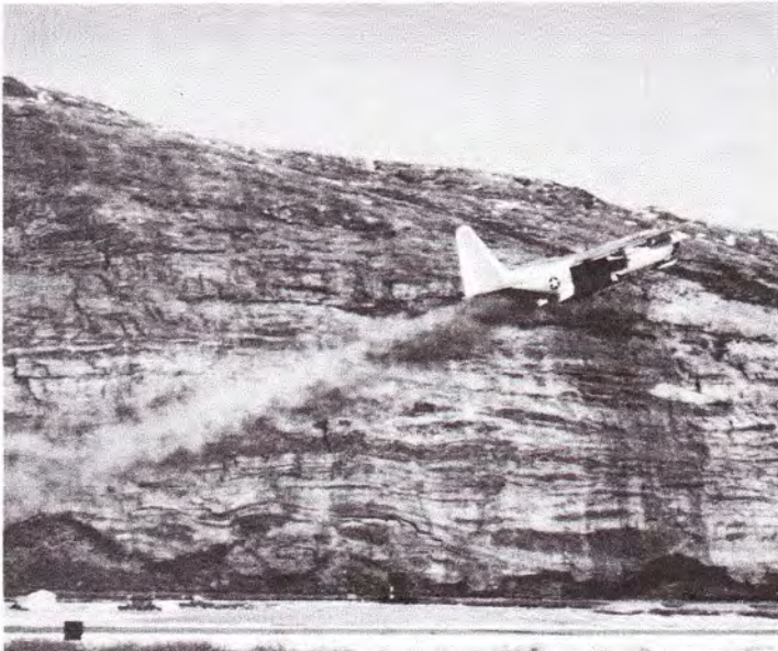
A C-130D makes a practice ATO assisted takeoff from the Sondrestrom AB runway. The practice is to familiarize pilots who sometimes have to use the system to literally blast themselves off the Ice Cap. (Author's Photo)
