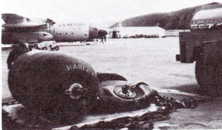
Before they switched to KC-97 fuel tanks, the Air Force used 500-gallon bladders to deliver diesel fuel to the sites. The bladders were strapped to pallets which were offloaded at the sites—a time-consuming job. (USAF Photo)
