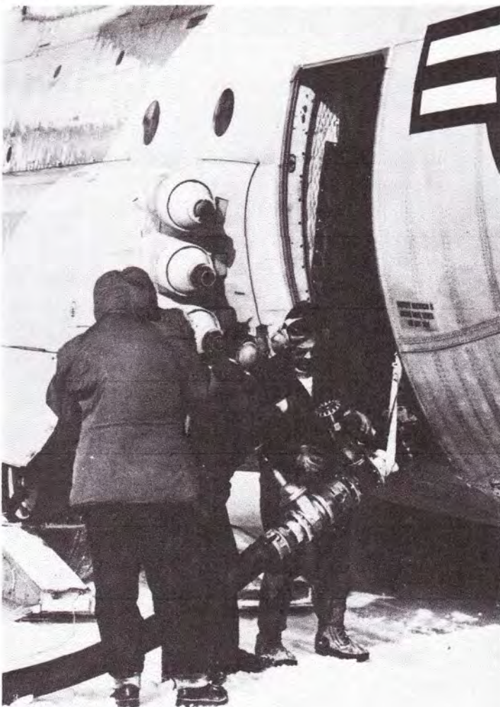
END OF THE LINE—A 17th Tactical Airlift Squadron loadmaster and two DYE site personnel unload fuel from a C-130 Hercules. The fuel is drained from tanks strapped to the cargo bed of the aircraft into storage tanks buried beneath the ice. Assisted takeoff (ATO) bottles are attached to the aircraft just forward of the door. (USAF Photo)
