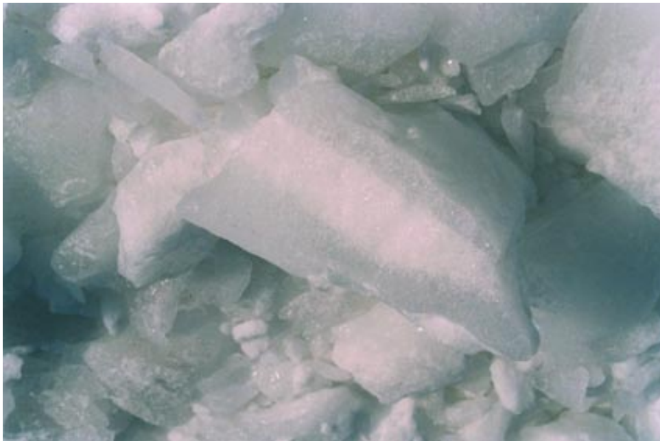
Figure 41. Poorly consolidated ice including snow pockets.
