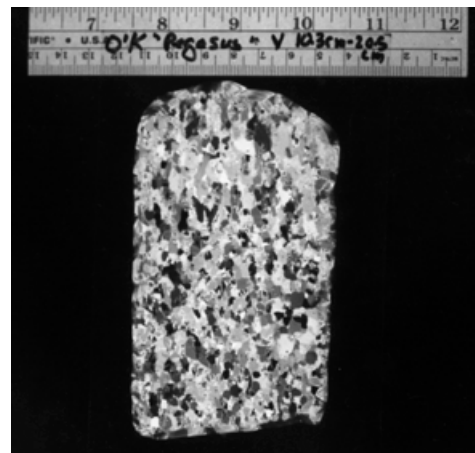
Figure 57. Horizontal and vertical thin sections at 10.3- to 20.5-cm horizon of core sample removed from the Pegasus runway surface at the 0-ft zone (north end).
