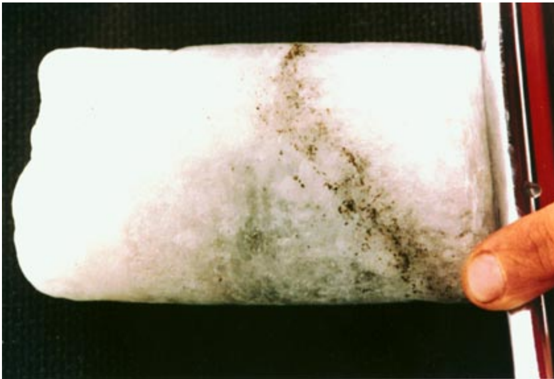
Figure 15. Mineral deposits in concentrated bands in ice.
