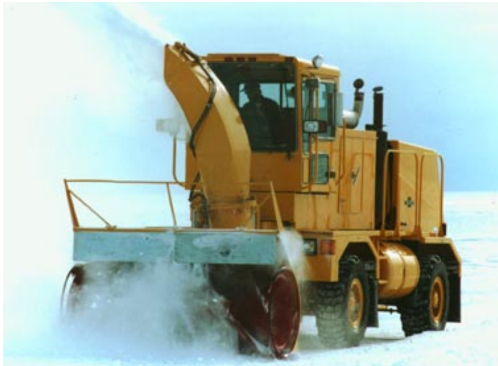
Figure 31. Rolba ribbon-type snowblower mounted on Oshkosh truck.
