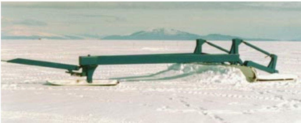
Figure 70. Medium snow plane with height and blade attack angle adjustability.
