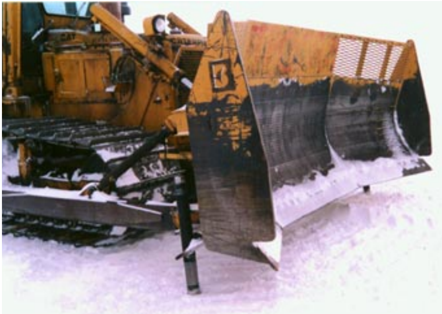
a. Skids installed on D6 bulldozer.
