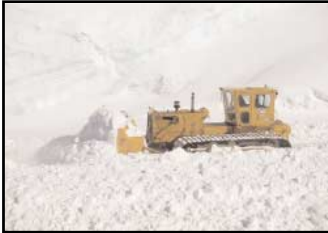
Photo courtesy of Larry Cook An older model Challenger D-8 tractor clears snow near McMurdo Station. The bulldozers have a wider track than newer models, making them more suitable for such work.
